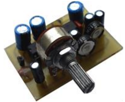
Photo 9. The headphone monitor module (without the rotary pickup selector switch)
