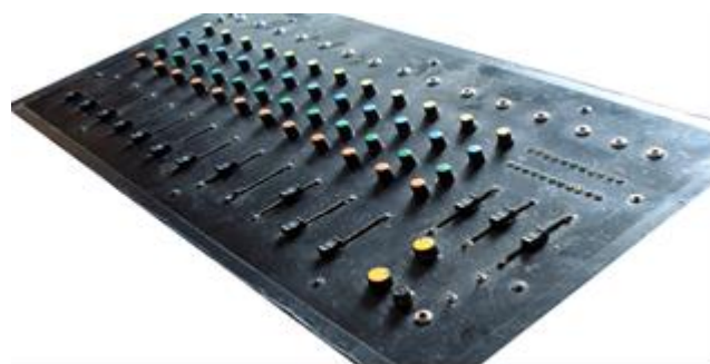
Photo 6. This prototype has 12 inputs and uses 3-bands tone control modules at all of them.
