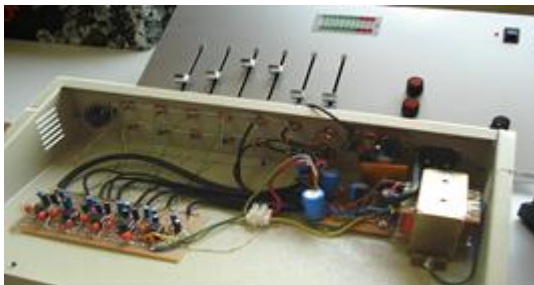
Photo 4. The mixer uses the modular-design concept. However, building some modules on the same board minimizes the number of cable connections required.
