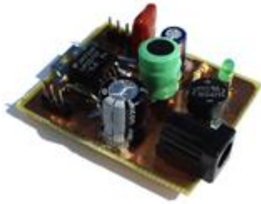
Photo 10. The small PSU, used to power the VU-meter
