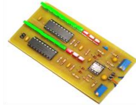
Photo 8. A bar-graph LED volume unit (VU) meter module, based on LM3915 IC
