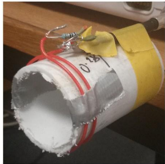
Figure 16. The coil antenna used by the research group at Surrey University [9].
