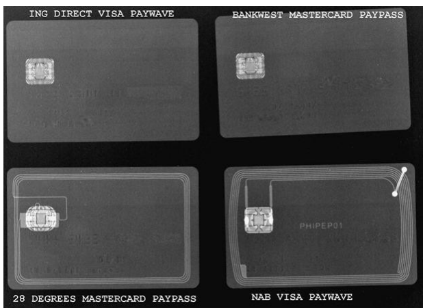
Figure 4. X-ray photos of four different NFC payment cards. [22]
